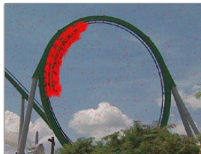
The red overlay helps to show which parts of the image have temporal recursive noise reduction applied.
